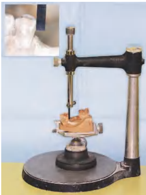
FIGURE 2-2 Dental cast surveyor facilitates the design of a removable partial denture. It is an instrument by which parallelism or lack of parallelism of abutment teeth and other oral structures, on a stone cast, can be determined ( magnified view shows parallel guide plane surface ). Use of the surveyor is discussed in later chapters.
