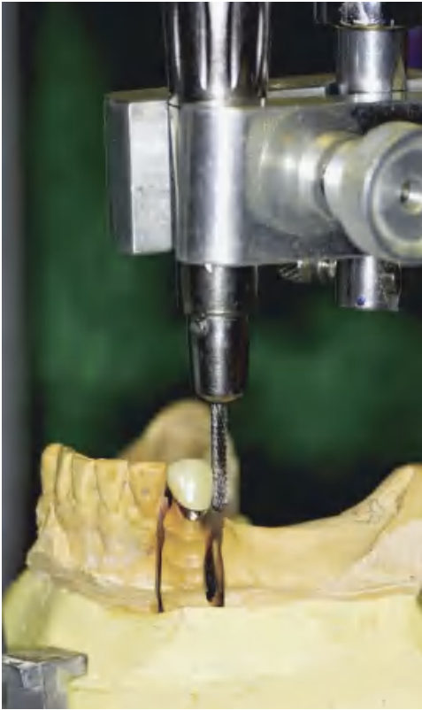
FIGURE 11-4 Lab handpiece clamp. Handpiece holders attach to the vertical spindle of surveyors and may be used to create and refine any parallel surface on a surveyed crown, as a drill press to prepare internal rests and recesses in patterns and/or castings, and to establish lingual surfaces above the ledge that are parallel to the path of placement in abutment restorations.
