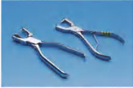
Figure 3.6 The traditional punch for making holes in rubber dam is the Ainsworth pattern (left). This incorporates a rotating wheel, which allows the selection of different hole sizes. Unfortunately, because of its complexity, this punch often deteriorates rapidly with repeated sterilization. This, coupled with the fact that one size of hole is usually adequate for most situations, has led the authors to adopt the much simpler Ash pattern punch (right) for routine use. This has the added advantage that the jaws can be removed and replaced at minimal cost if they become damaged.
