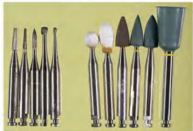
Figure 5.32 Finishing burs, stones, and points for dental amalgam. From the left: five plain-cut latch-grip steel finishing burs, two mounted white (alundum) stones, three mounted abrasive rubber points from coarse to fine, and a mounted abrasive rubber cup.
