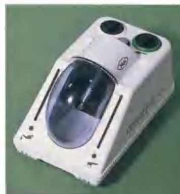
Figure 5.7 An automatic handpiece cleaning unit which is connected to the air supply. The shield at the front is rotated out of the way and the handpiece plugged onto the connector. A detergent is then flushed through the handpiece followed by oil, both of which come from refillable containers at the back of the unit. This is a more efficient and quicker system than using aerosols.
