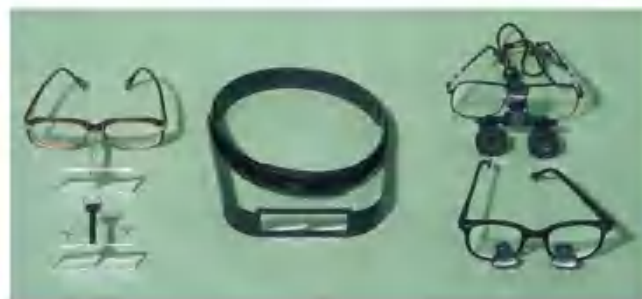
Figure 5.19 A selection of magnification loupes. The first three are the cheapest and have the simplest optics, clipping onto existing spectacles/safety glasses or being secured with a head loop. The two on the right are more expensive. The top right pair have interchangeable lens blocks and due to their weight, require a head cord for retention. Those on the bottom right have the dentist's fixed interpupillary distance built in as the lenses are cemented through the prescription/safety spectacle lenses. As the magnification optics are closer to the eye, this results in a greater field width and depth of field but at increased expense.
