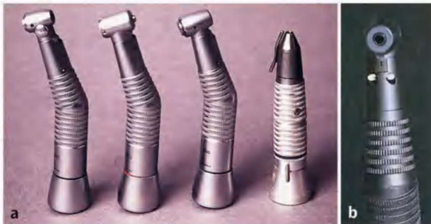
Figure 5.29 (a, b) A selection of low-speed handpieces. From the left: 1:1 contra-angled handpiece used for most procedures. Latch-grip burs are used. Commonly identified with a blue-coloured band on the shank of the handpiece and a blue dot on the head. Speed in the range 400–40 000 rpm. 1:4 speed-increasing handpiece. Friction-grip burs. Operates at 16 000–160 000 rpm. Commonly identified with a red band. Useful for finishing cavity preparations and also finishing restorations. 7:1 speed-reducing handpiece. Latch-grip burs. Used for drilling pin holes and other procedures where slow speed is indicated. Operates at 550–5500 rpm and is commonly identified with a green band. Straight handpiece that takes straight burs (may be modified to take latch-grip burs). A 1:1 handpiece is identified with a blue band; speed-reducing is identified with a green band. Used to trim temporary restorations and other similar procedures. Usually used outside the mouth. A fibreoptic light system built into the head of a contra-angled low-speed handpiece.
