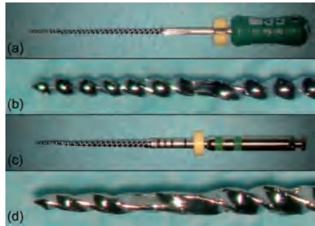
Fig. 11.23 (a, c) Hand and rotary files showing unwinding of the flutes. (b, d) A detailed view on the area with deformation.
