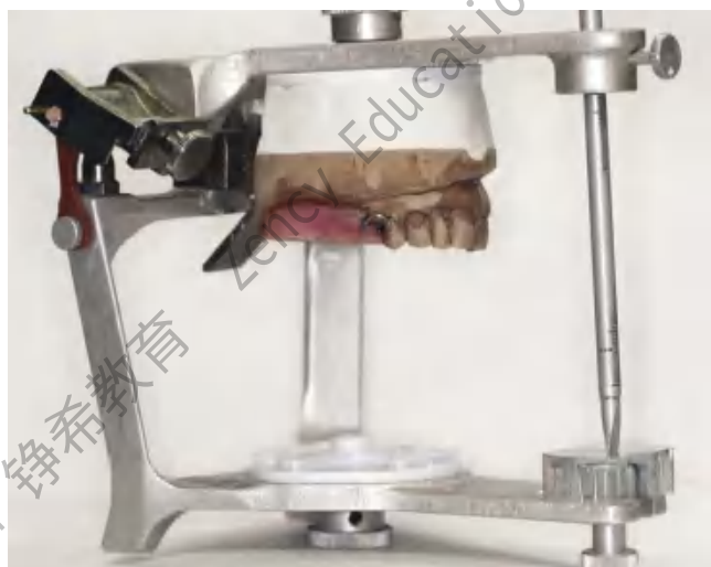
FIGURE 12-11 Facebow mounting is complete. The relationship of the maxillary cast to the articulator condylar components is anatomically similar to that between the patient's maxilla and the bilateral temporomandibular joint (TMJ) complex. Any subsequent tooth arrangement and occlusal contact development will represent the mouth more accurately than more arbitrary mountings. The benefits of the anatomic similarity are seen in more accurate occlusion for the finalized prosthesis (i.e., less intraoral adjustment required).
