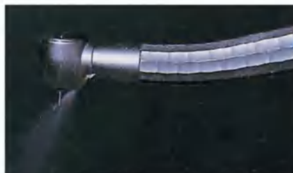
Figure 5.28 Air turbine handpiece in operation showing the directed water spray over the tip of the bur and the fibreoptic light.
