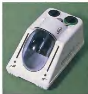
Figure 5.7 An automatic handpiece cleaning unit which is connected to the air supply. The shield at the front is rotated out of the way and the handpiece plugged onto the connector. A detergent is then flushed through the handpiece followed by oil, both of which come from refillable containers at the back of the unit. This is a more efficient and quicker system than using aerosols.
